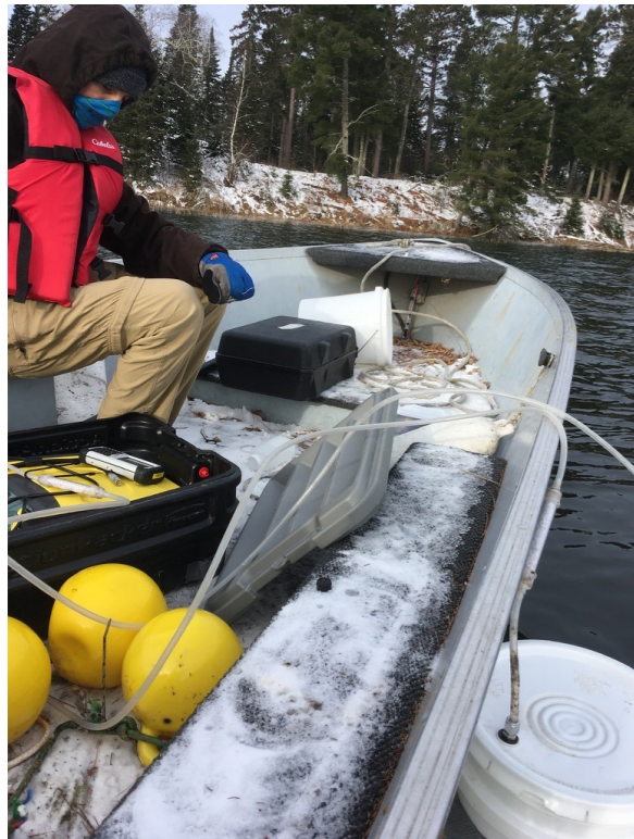
The FTIR system for measuring CO 2 , CH 4 and N 2 O. This portable instrument consists of a chamber that floats on the water and the FTIR instrument (yellow instrument in black box).
