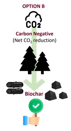
Carbon in trees is transformed into biochar which is stable and unsusceptible to microbial decomposition.
