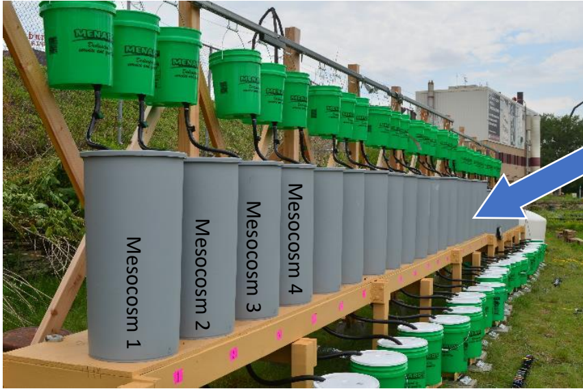
Experimental mesocosm setups to test CEC removal efficiency of different engineered media. Location: St. Anthony Falls laboratory (photo courtesy B. Heitkamp)
