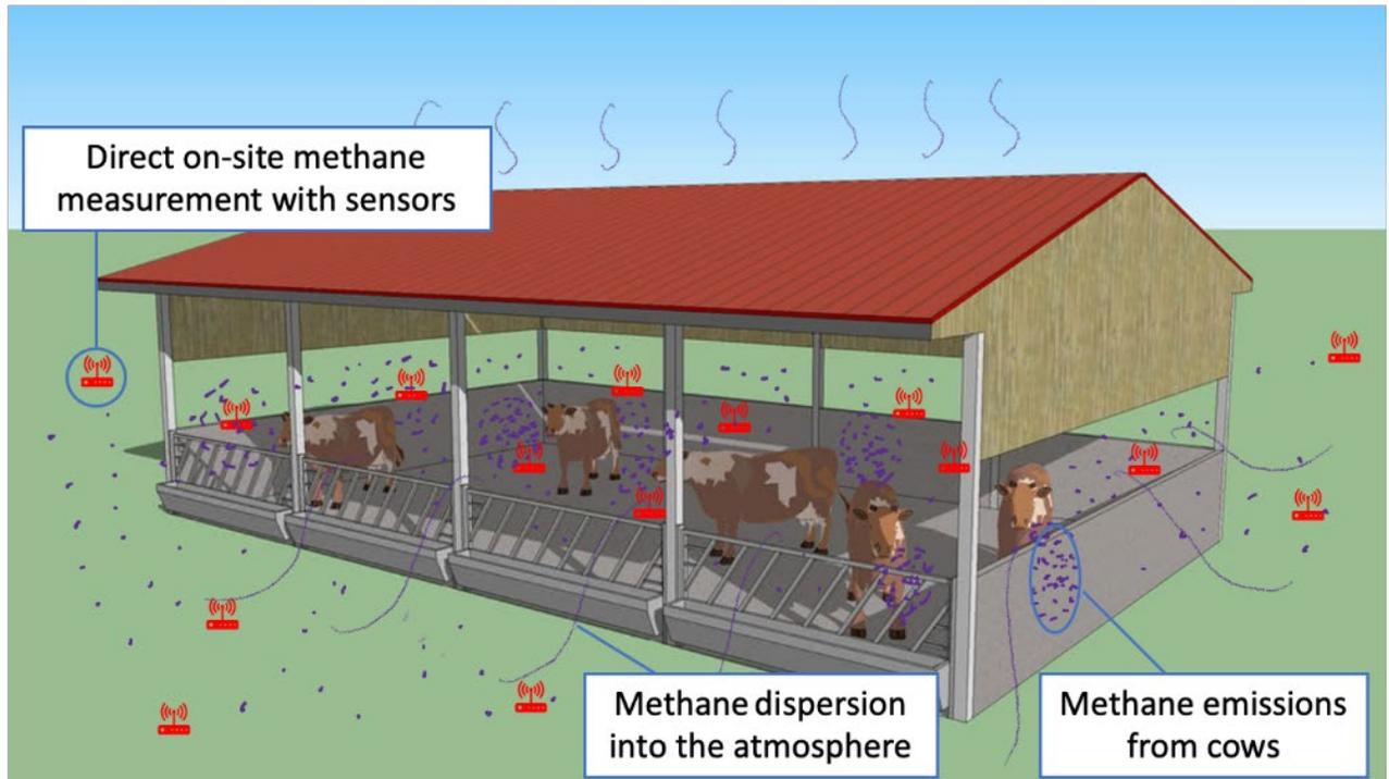
(2) The low-cost sensor suite in development for methane detection
