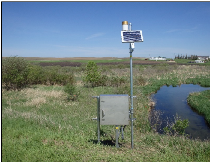
Example of installed wetland hydrology monitoring station.
