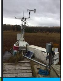
Methane and carbon dioxide fluxes between the peatlands and the atmosphere will be measured on unrestored and restored peatlands using "eddy flux" towers like this one run by us in a Minnesota peatland.
