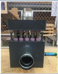
Non-thermal plasma (NTP) reactor for AIV inactivation being developed at UMN Sanitized air
