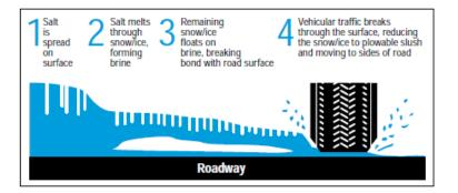
Replace inefficient spreading of salt (large quantities, slow reaction rate)
