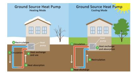
A geothermal system uses the relatively stable deep ground temperature to provide cooling in summer and heating in winter with high coefficients of performance<sup>1</sup>.
