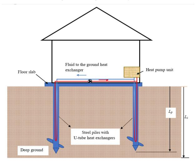
A heat pump coupled to a thermo-active helical steel pile type building foundation using u-shaped heat exchanger. This is the conventional heat exchanger system, enhanced heat exchanger systems will be developed and optimized and their performance compared with the standard u-loop heat exchangers.
