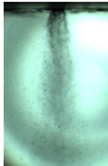
Atomization/combustion of viscous liquid
