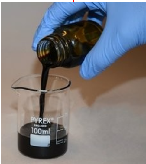
Viscous suspension of fuel in glycol/glycerol
