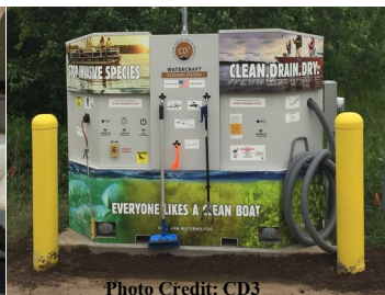
Visual inspection and cleaning station tools (e.g. tongs, air blower, vacuum, and scrub brush)
