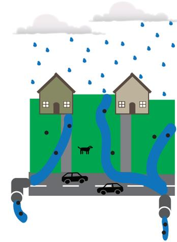
Various infiltration practices are used to reduce the volume of stormwater directly entering nearby surface waters.
