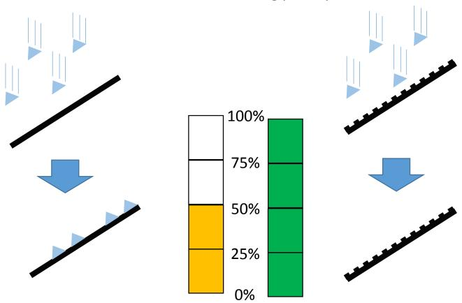
Contamination falling on untreated panels sticks and reduces electrical output. Page 5 of 6
