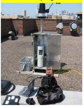
This type of air sampling separates airborne particles by size for characterization, and retains an archive of those particles for future ENRTF ID: 181-E
