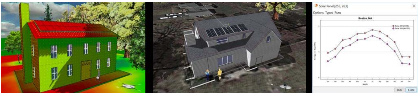
Figure 1. Example house with solar panels and intensity of solar radiation shown in color, house superimposed on google maps, and model results showing energy generated by solar panels. Source: http://energy.concord.org/energy3d/projects.html
