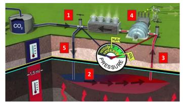
CPG system design when circulating  $CO_2$  through the deep subsurface.
