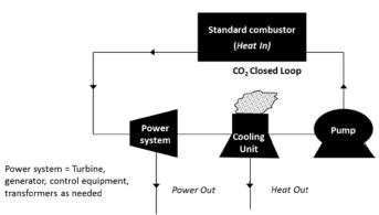
Closed-cycle CO<sub>2</sub> power system design for the proposed project. The simulated geothermal energy source will be used to test the innovative power system over a variety of anticipated field conditions.
