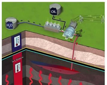
CPG system design for first field tests, where old oilfield infrastructure is repurposed for geothermal power generation using a closed-cycle CO<sub>2</sub> power system.
