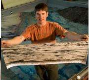
☆A SAFL graduate student holds a crosssectional 'peel' of sediments deposited in an experimental delta.
