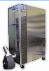
Non-thermal plasma reactors for animal housing air treatment
