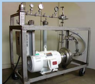
Concentrated high intensity electric field (CHIEF) system for liquid treatment
