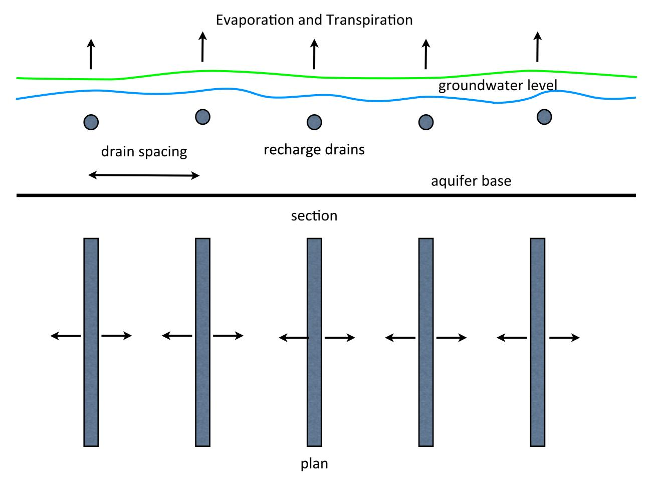
Using recharge drains to invigate crops from below.
