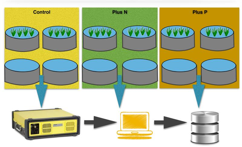
A portable gas analyzer similar to this one, will be used to quantify methane,  $CO_2$ ,  $N_2O$ , and  $NH_3$  as well as other important greenhouse gases and dissolved nutrients. In addition, we will deploy oxygen and temperature sensors in each artificial mesocosm. Data will be analyzed, curated and placed in our online database.
