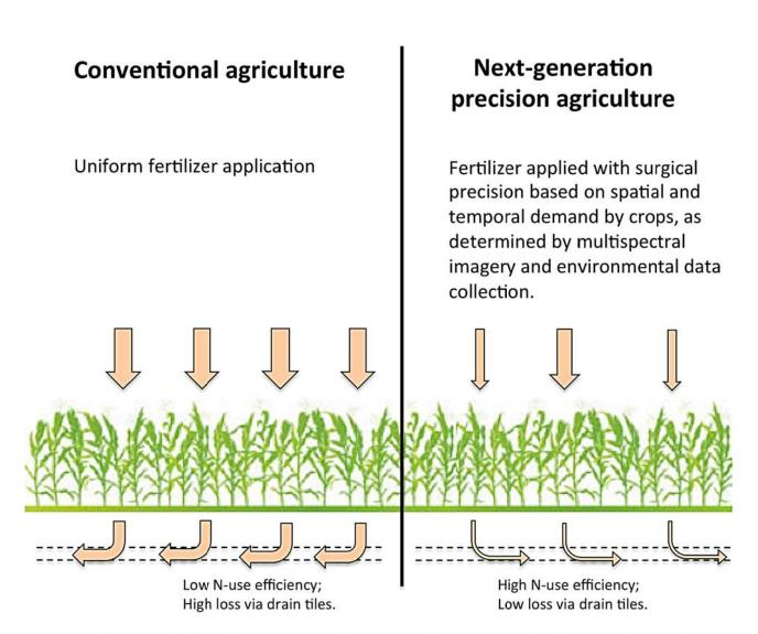
We will quantify the changes in yield, N-use efficiency, and N loss via drain tiles, from corn produced using next-generation precision agriculture compared to conventional management.
