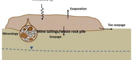
C. Theoretical waste rock or tailings pile, showing factors addressed in this study that contribute to the quantity and quality of water leaving the pile.
