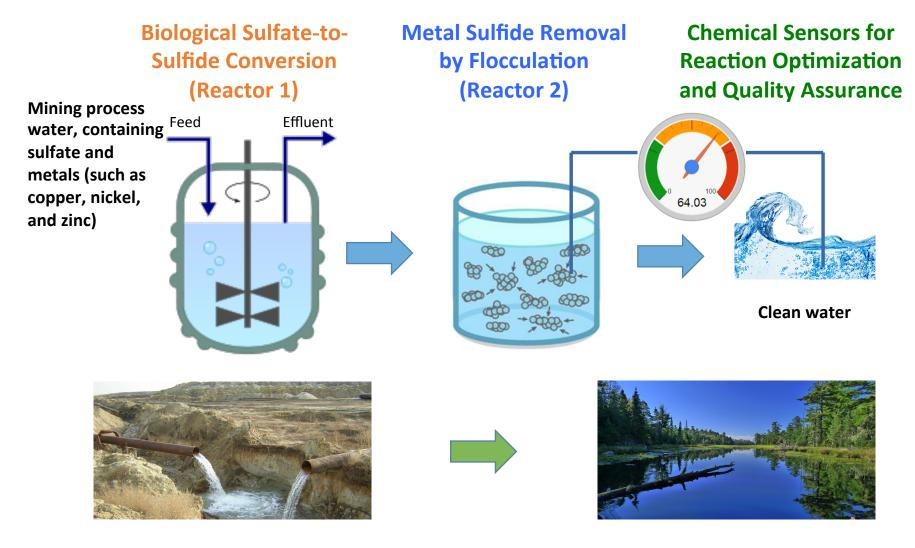
In reactor #1, sulfate is reduced by bacteria to sulfide, which helps precipitate heavy metal contaminants. The sulfidemetal particles are removed efficiently in reactor #2 using an organic polymer surfactant, permitting metal recycling. Use of on-line chemical sensors minimizes waste and assures the quality of the cleaned water.
