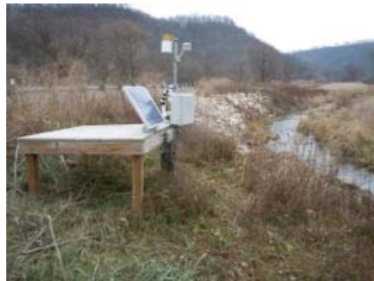
Water monitoring station on Garvin Brook.
