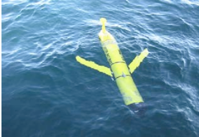
Underwater autonomous glider for mapping sediment and colored dissolved organic matter inputs, and biological responses.
