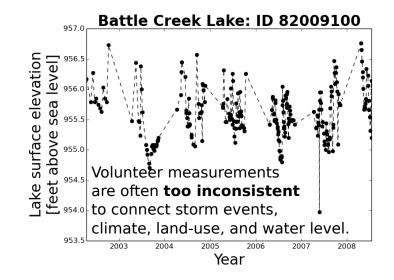
**Top:** High-quality scientific predictions require consistent and frequent data that lets us connect storm events, climate, and land-use to lake levels. **We propose to couple new automated sensors with groundwater probes that tell us how lakes provide water to or draw from groundwater aquifers.**
