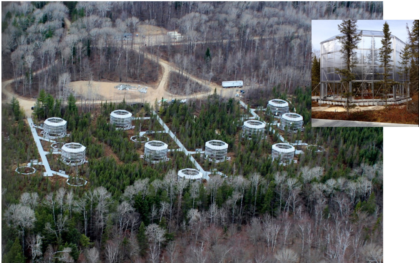
Aerial view of the SPRUCE Project and the 10 environmental enclosures located on the S1 bog at the Marcell Experimental Forest north of Grand Rapids, MN. The inset is a ground view of one of the enclosures as construction nears completion.
