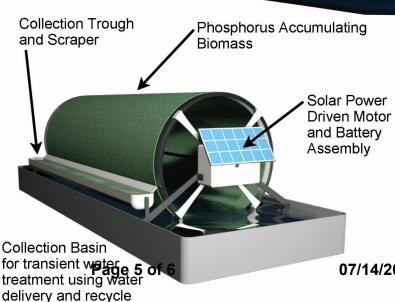
Modular Design will allow the reactor to be applied to various environments by making minor modifications. Shown above is a floating reactor scheme. Combined with various sensors and "smart" technologies, this reactor could be directed to regions high in phosphorus, and would navigate back to a dock to empty excess biomass when the system reaches capacity. In place reactors (left) can be used to cycle water from small ponds or streams for temporary treatment, and could be set up in series.
