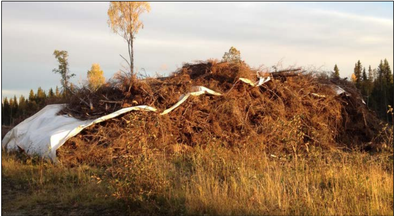
Figure 1. Biomass pile with paper cover in Östersund, Sweden after nine months drying (September 2013).
