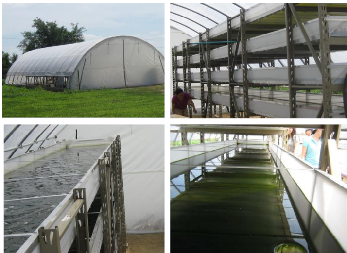
Figure 2. Pilot scale animal wastewater algae production facility in Rosemount, developed through previous LCCMR and other projects.
