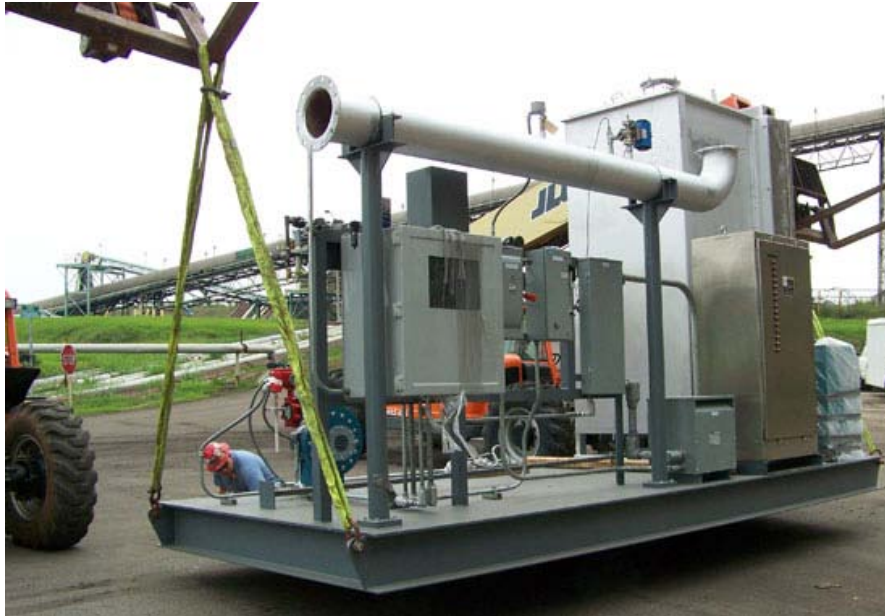
Fig.1: Pilot unit skid for lignite coal-fired power application
