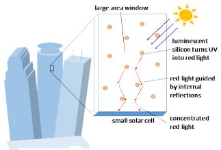
Figure 1: Schematic of a solar concentrator window
