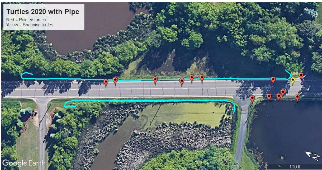
Figure 5. Site S1 before (top) and after (bottom) pipe barrier installed. Barrier indicated by blue lines. Turtle mortality was dramatically reduced from 2019 to 2020 after the barrier was put in place. Note that some turtles still have access to the roadway from a pond in the southwest where a barrier could not be installed.
