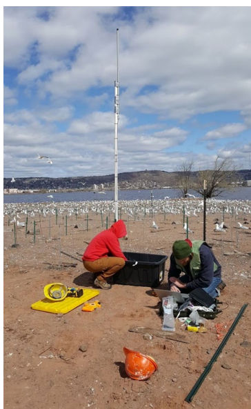
Figure 2.1. Omnidirectional Motus station placed on Interstate Island on May 30, 2019. This station is listening for and recording signals from radio transmitters placed on Common Terns breeding at the island 24hr/day.
