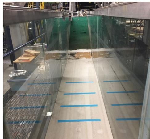
Figure 4. Photo of the interior of the wave flume. Stripes of colored sand were used to observe the onset of sediment movement.
