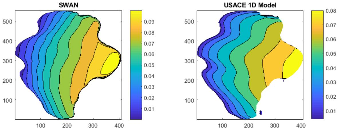
Figure 12. Simulated significant wave heights on Belle Lake for a wind event on Oct 4, 2017, with mean wind speed of 4.2 m/s at 285° CCW from the north. SWAN was used with wave setup Model B, with wind distributed on the lake per fetch distance predicted by the USACE model and wind speed reduction from roughness transition at the shore per Taylor and Lee (1984).
