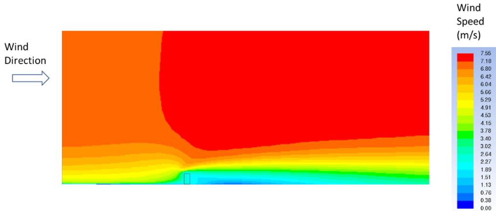
Figure 9. Two-dimensional simulated velocity field for wind flow over a line of trees adjacent to a pond or lake, showing the wind sheltering (speed reduction) downwind of the tree line. ANSYS-Fluent is being used for the simulations.
