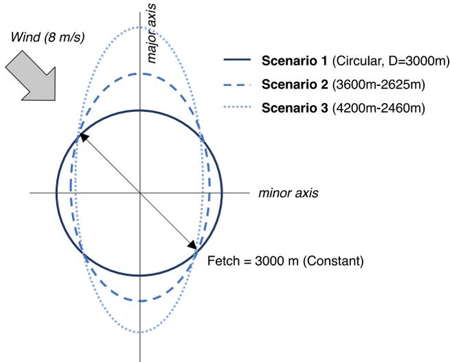
Figure 17. Schematic of lake geometries used to test wave refraction in lakes with irregular (oblong) shapes. Scenarios set up so that wind-aligned fetch (NW-SE) had a constant distance of 3000m among scenarios. Wind constant from NW at 8 m/s.
