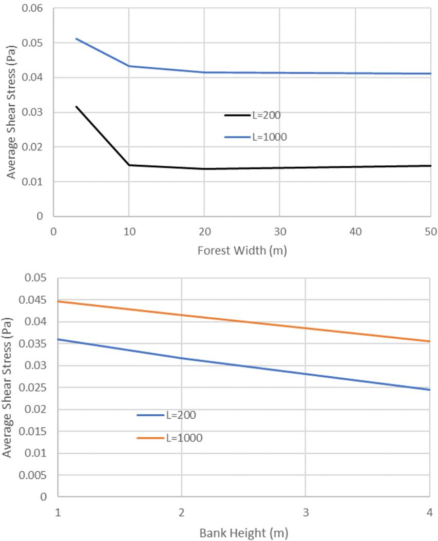
Figure 11. Average shear stress over a water body versus the width of the adjacent forest strip (upper panel) and average shear stress versus bank height (lower panel for 200 m long and 1000 m long water bodies).
