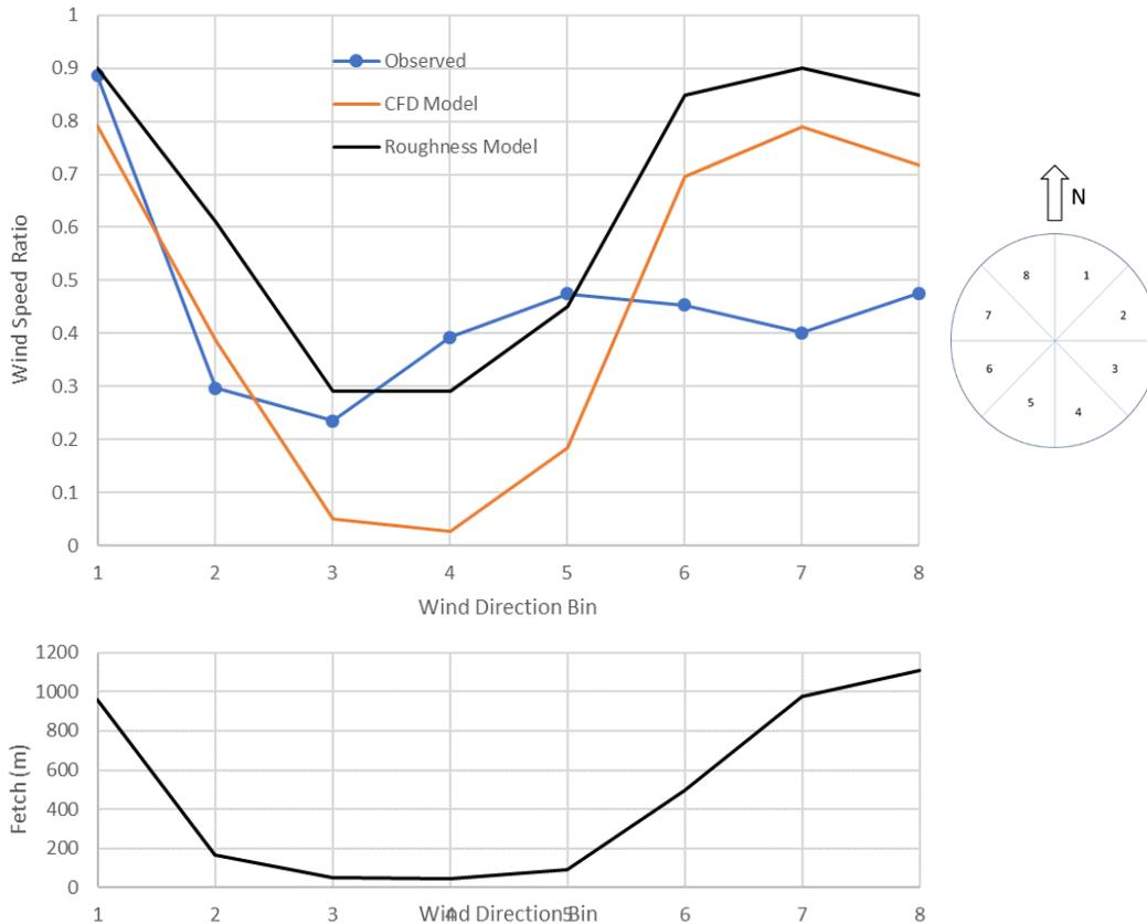
Figure 19. Observed and simulated wind sheltering (wind speed ratio) for Swan Lake (upper panel) and wind fetch versus direction (lower panel). The wind direction bins are numbered 1 through 8, as shown in the diagram to the right.
