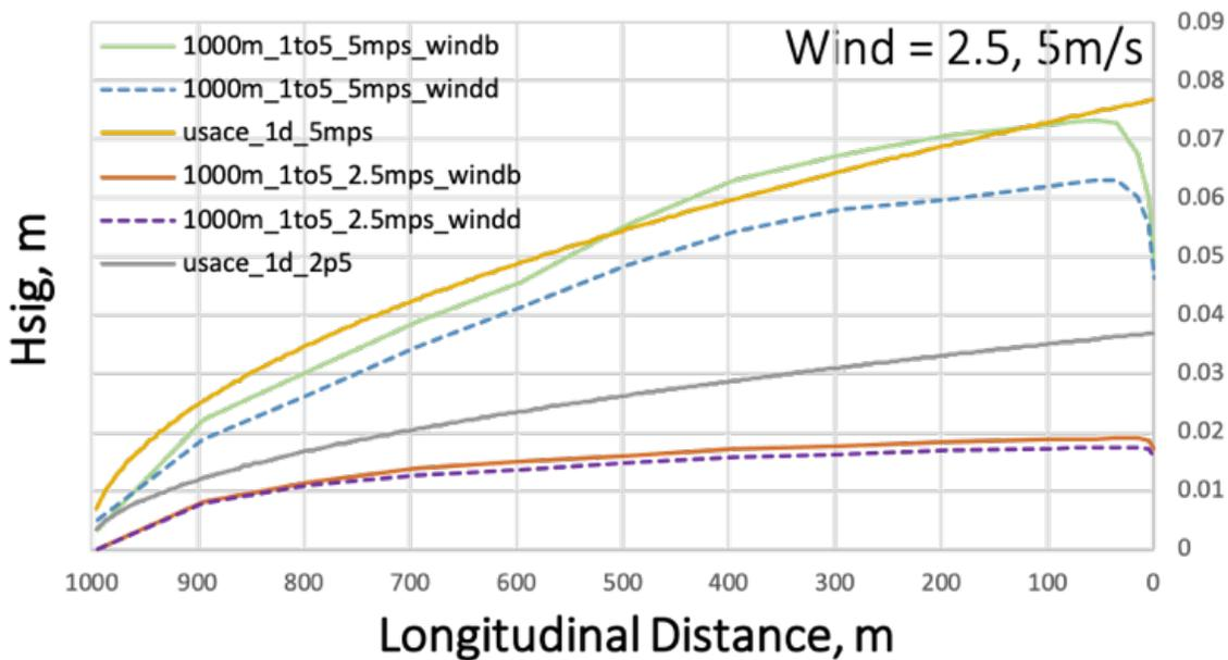
Figure 13. Comparison of significant wave height predictions from SWAN models B and D vs. USACE 1-D wave model for a 1000m-long domain for wind speeds of 2.5 m/s and 5 m/s wind speed. Note the larger differences in open water wave height prediction at low wind speeds (2.5 m/s).
