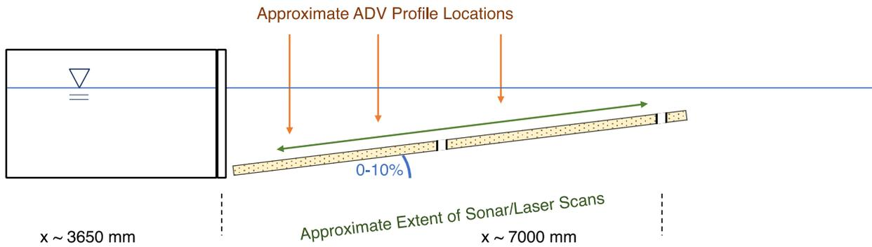
Figure 14. Schematic of SAFL wave flume with adjustable-slope bed. Wavemaker apparatus located off-diagram to the left at a location of roughly  $x=1000\text{mm}$ . Rock was placed at the upslope end of the adjustable bed where it met the fixed ramp (“beach”) to prevent unrealistically high scour from occurring at the abrupt junction.
