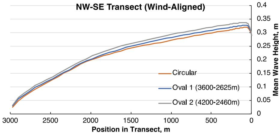
Figure 18. Simulations of mean wave height (m) versus position using the 2-D SWAN wave model along the wind-aligned direction.
