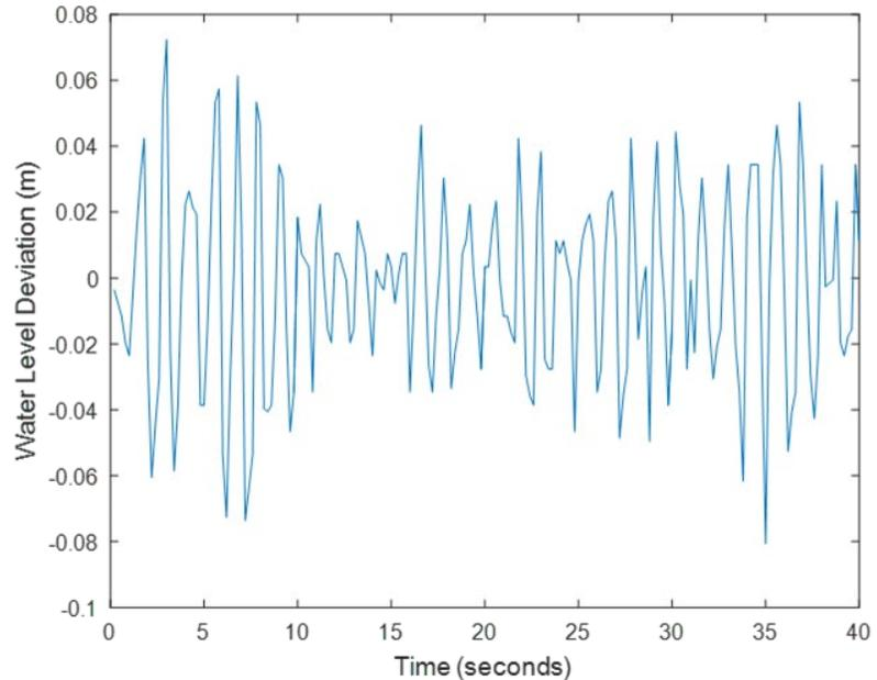
Figure 1. Left Panel: A photograph of the wind/wave measurement station installed in Belle Lake, showing the data logger, solar panel, and wind measurement instrumentation. The water level sensor is mounted beneath the data logger box, and is not visible. Right panel: A 40 second sample of the water level data taken at the station on October 15, 2017, with wave amplitudes of up to 0.13 meters (0.43 feet) driven by wind speeds of 5 m/s (11 miles per hour).
