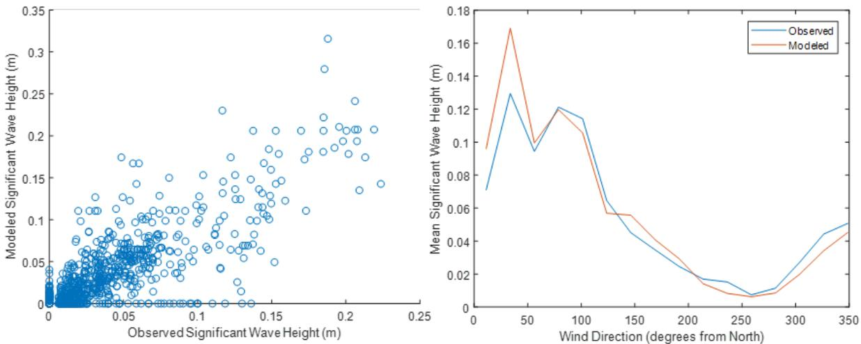
Figure 3. Comparisons of modeled and observed wave height on Ten Mile Lake, Sept 21 to Nov 1, 2018. Left Panel: Modeled versus observed mean hourly wave height, for all wind directions. Right panel: Modeled and measured mean wave height versus wind direction.
