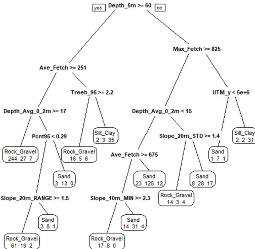
Figure 7. Classification tree for predicting the substrate size classes.
