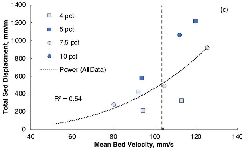
Figure 16. (a) Observed vs. Modeled bed velocity for all measurement locations across experiments (0% - 10% slope) with the fine sand (median diameter 0.1 mm), binned by water depth; (b) Local sediment displacement (mm; estimated from sonar) vs. observed bed velocity; (c) Total sediment displacement along the slope (mm displacement per m of slope) vs. mean observed bed velocity, with each point representing a given scenario of wave and slope conditions (lowest wave height scenarios omitted).
