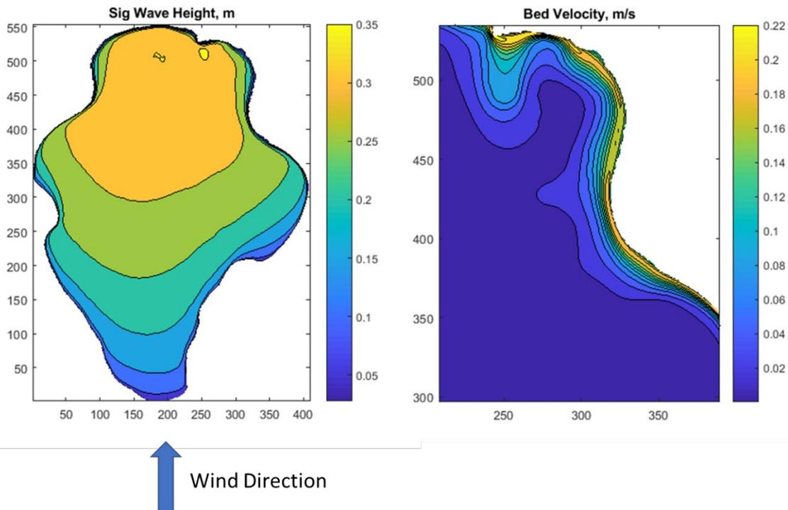
Figure 8. Sample output from the 2D wave model (SWAN) for Belle Lake, including a map of the significant wave height over the lake and a detail of the predicted nearshore bed velocity.
