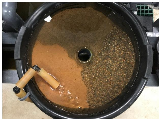
Images 9 (left) and 10 (right): (9) Pans are set-up with silt, sand, pebble, and mixed substrate types. (10) The mixed substrate pans included relatively equal amounts of the three grades of substrate (shown prior to mixing).
