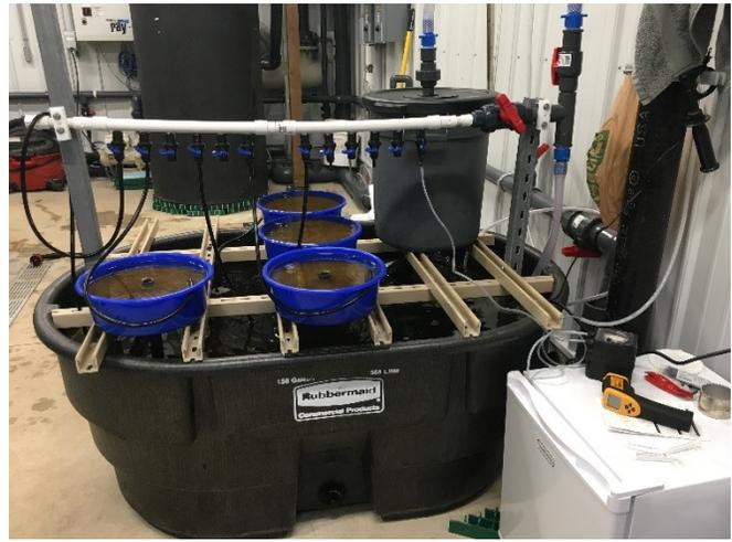
Images 7 (left) and 8 (right): (7) New propagation and research systems were installed this winter and are now operational. (8) A quarantine system to evaluate condition of newly acquired mussels and identify and remove unwanted species was also installed. A pump delivers food regularly in this system to simulate the near constant supply of food that would exist in the wild.
