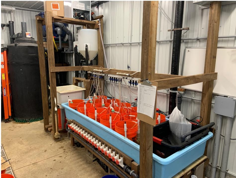
**Image 23:** The surge bucket system allows for automated water changes in the buckets to provide new food and remove animal waste, creating optimal rearing conditions for newly transformed mussels.
