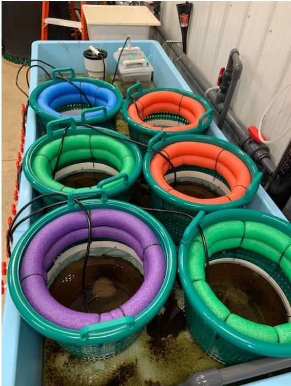
**Image 13:** New trough system installed in mussel research facility with novel rearing tank prototypes and basket systems being prepared to hold mussels from the DNR.
