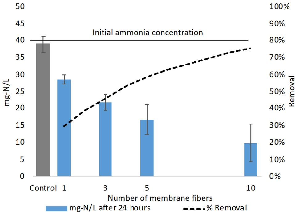
Figure 1.1. Ammonia removal from synthetic wastewater with zeolite coated alumina hollow fibers
