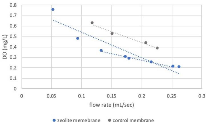
Figure 2.1. Result from oxygen-flux testing of zeolite and uncoated membranes in a flow-through system.
