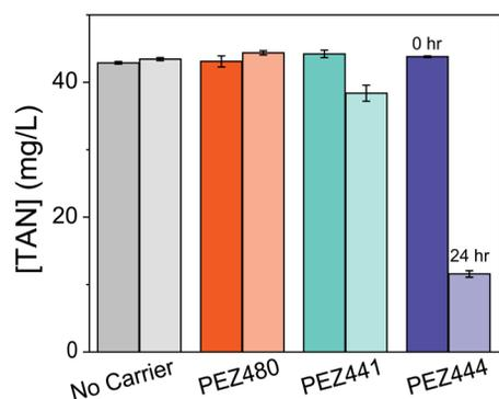
Figure 1.6. Ammonium removal from 45 mg/L ammonium solutions after 24 hours. The carrier labeled “PEZ480” contained no zeolite. The carrier labeled “PEZ441” contained a low quantity of zeolite and the carrier labeled “PEZ444” contained 45% by mass zeolite. The concentrations shown represent the average of three separate experiments, with the error bars representing the standard deviation.
