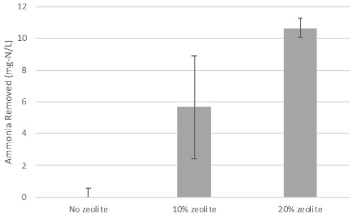
Figure 1.3. Ammonia removal after 24 hours by sorption to carriers containing different quantities of zeolite on their surface (no zeolite, 10% zeolite by mass, and 20% zeolite by mass).
