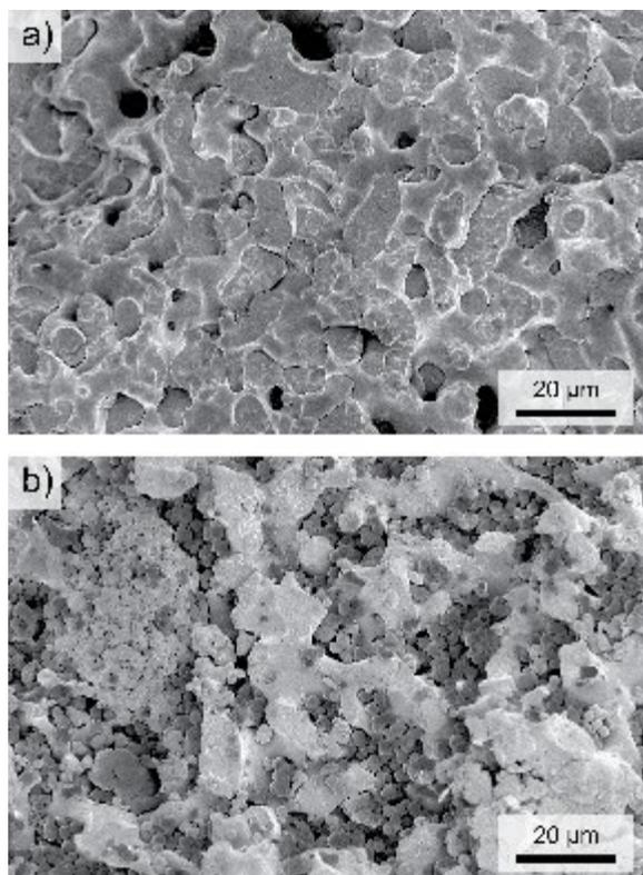
Figure 1.5. Scanning electron micrographs of the 45% zeolite carrier before (a) and after (b) solvent etching in water to remove the PEO template. The continuous pore structure with physically entrapped particulate zeolite (visible as small darker-toned particles) is clearly visible after etching.
