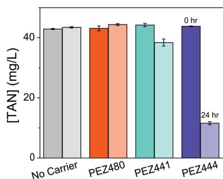
Figure 1.6. Ammonium removal from 45 mg/L ammonium solutions after 24 hours. The carrier labeled “PEZ480” contained no zeolite. The carrier labeled “PEZ441” contained a low quantity of zeolite and the carrier labeled “PEZ444” contained 45% by mass zeolite. The concentrations shown represent the average of three separate experiments, with the error bars representing the standard deviation.
