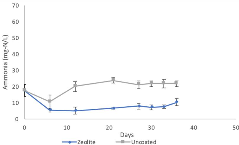
Figure 1.4. Ammonia effluent concentrations from experiments containing wastewater bacteria and either zeolite-coated or uncoated alumina hollow fibers. It can be seen that the zeolite-coated fibers removed significantly more ammonia than the uncoated fibers over the course of the experiment, which was a result of the stimulation of microbial ammonia removal.
