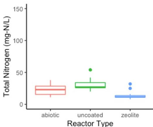
Figure 7. Effluent Total Nitrogen Concentrations from the batch reactor membrane experiments.
