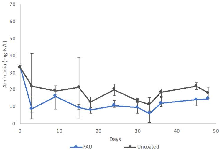
Figure 1.2. Ammonia effluent concentrations from biologically active batch reactors with zeolite-coated (labeled “FAU” for faujasite-type zeolites) and uncoated alumina hollow fibers. It can be seen that the faujasite-coated fibers removed more ammonia than the uncoated fibers over the course of the experiment.
