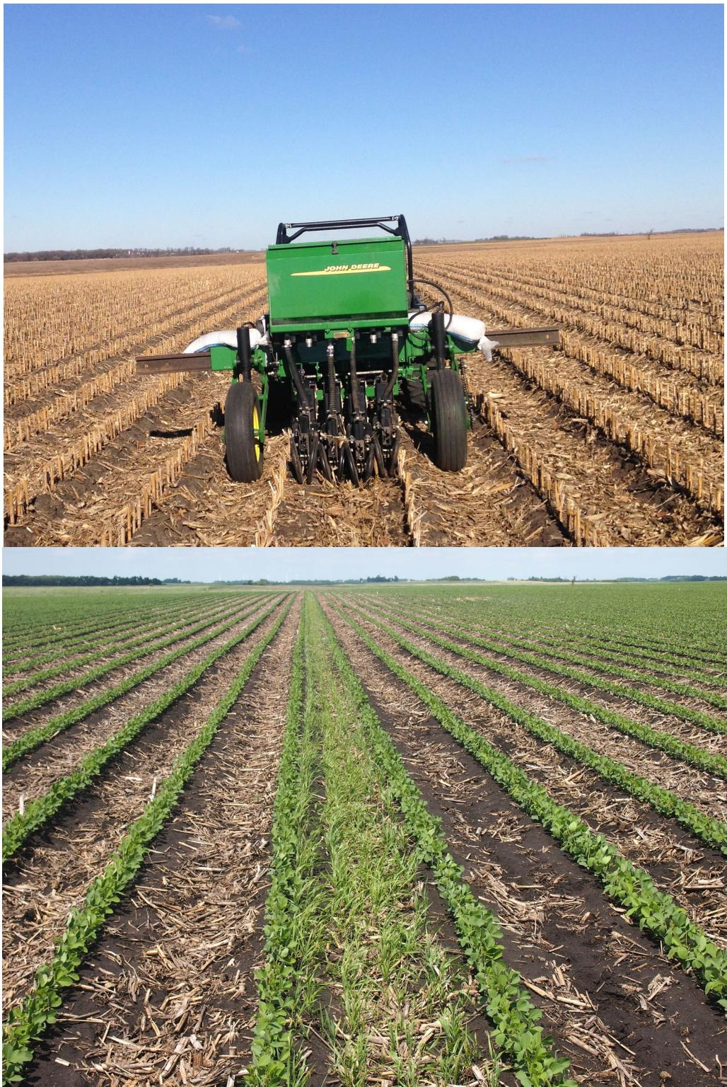
**Figure 1.** Upper : custom no-till seed drill designed to plant four rows in the 30 inch area between corn rows.
