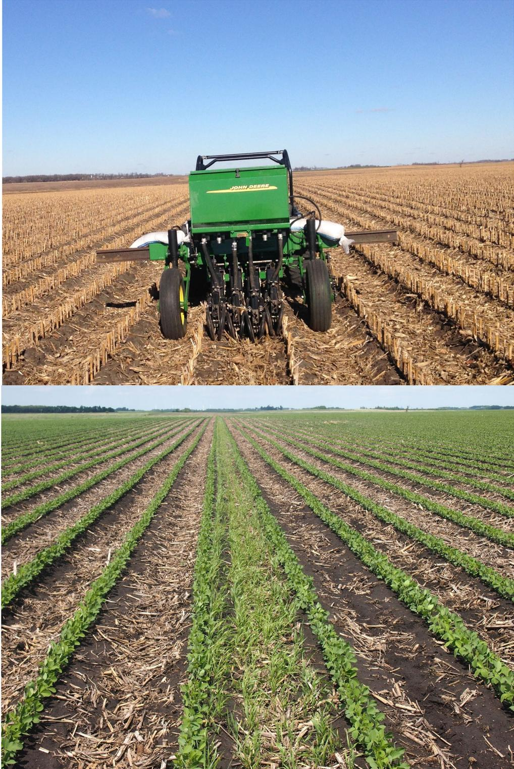
**Figure 1.** Upper : custom no-till seed drill designed to plant four rows in the 30 inch area between corn rows. Lower: Savanna grasses planted in November of 2016 and growing well between soy row planted in June of 2017.
