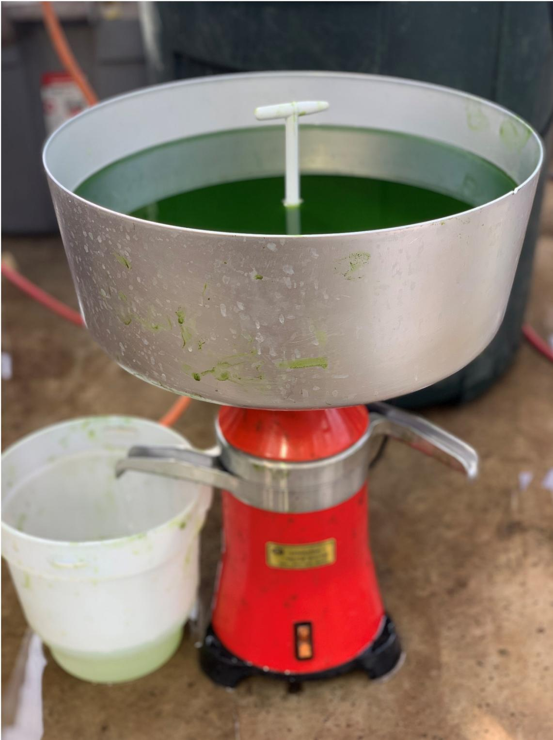
Figure 9. Cream milk electric centrifugal separator (version 100-18), Motor Sich JSC© used to separate the biomass and the liquid part from the bags containing dairy wastewater and water.
