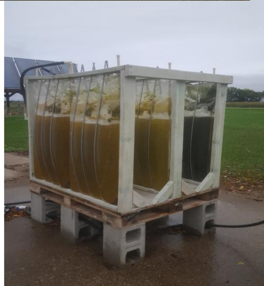
We have scaled up the algae bioreactor demonstration and have begun testing algae concentrations. Data analysis is in preparation.
