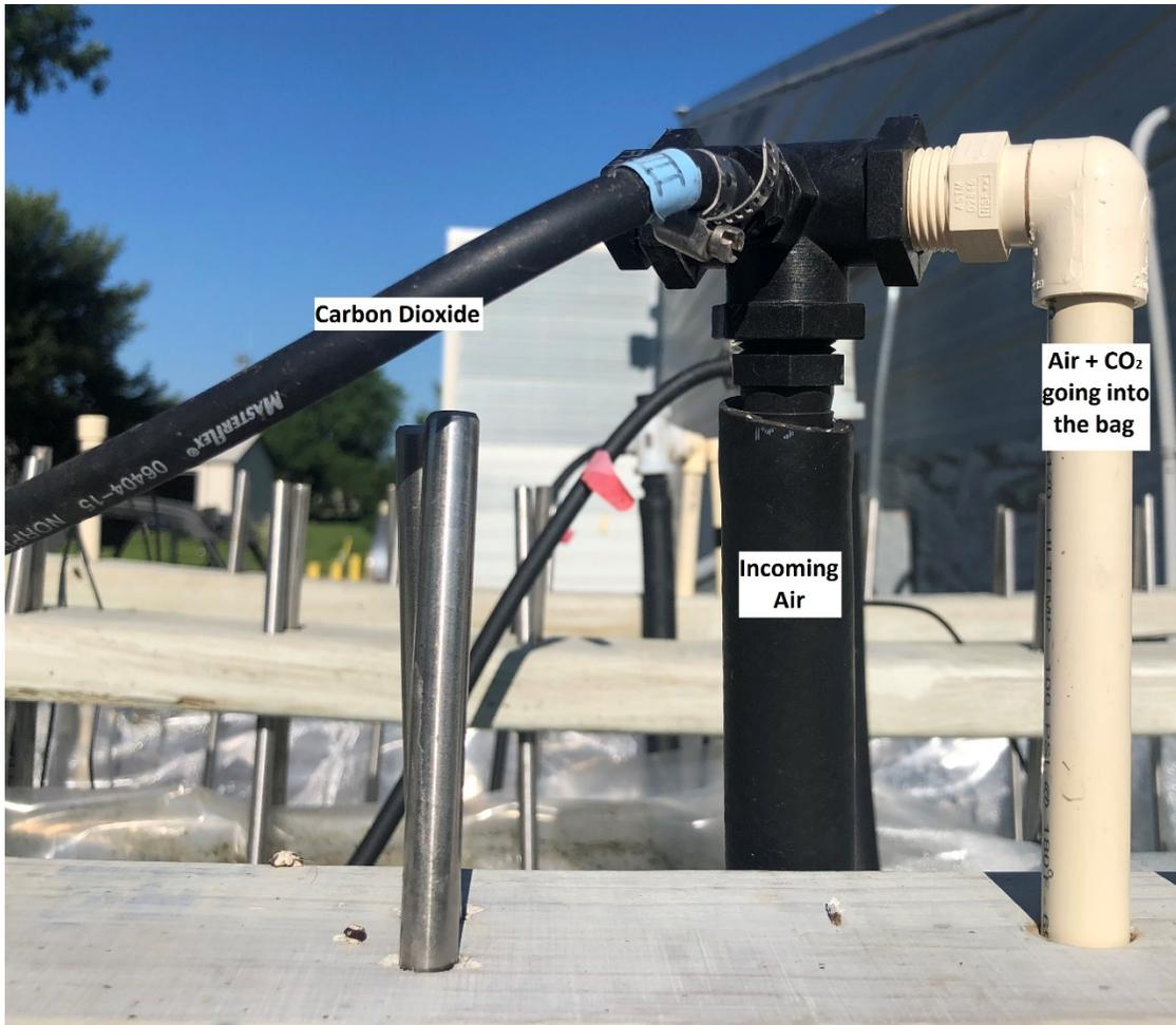
Figure 5. Detail on the air and carbon dioxide mixture going into the system.
