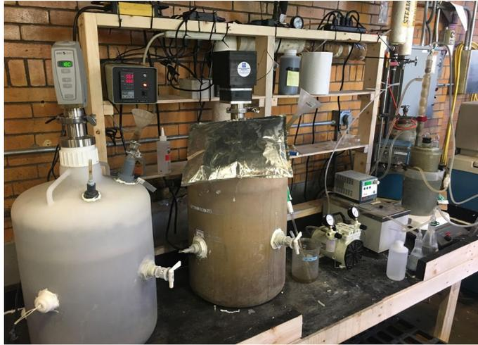
Figure 1. The experimental apparatus for thermophilic AD with light vacuum side to treat animal wastewater.
