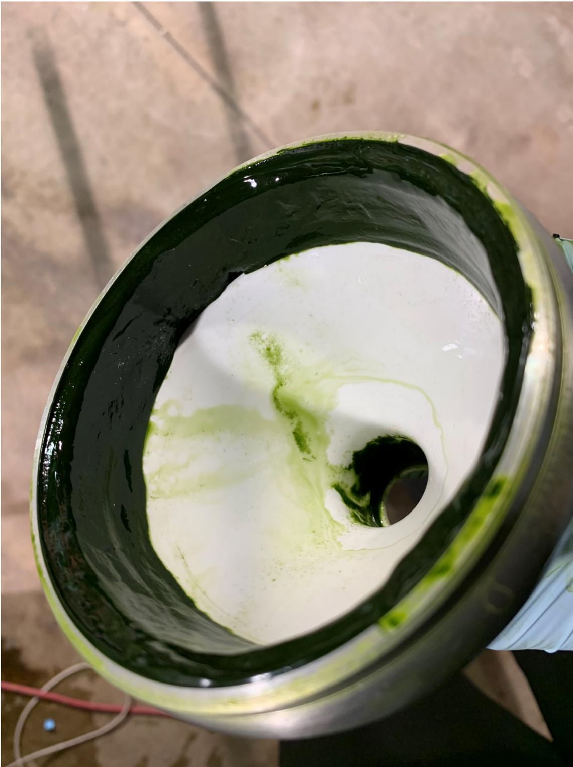
Figure 10. *Chlorella sp.* biomass collected inside the cream milk electric centrifugal separator (version 100-18), Motor Sich JSC©.
