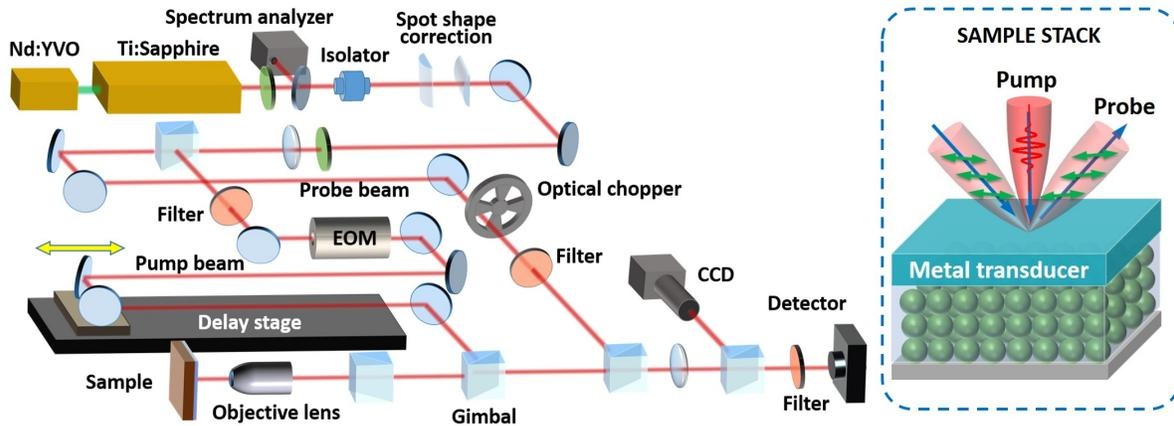
Figure 4: Schematic of the custom-built ultrafast pump-probe system and the Si-Ge sample stack for thermal measurements.
