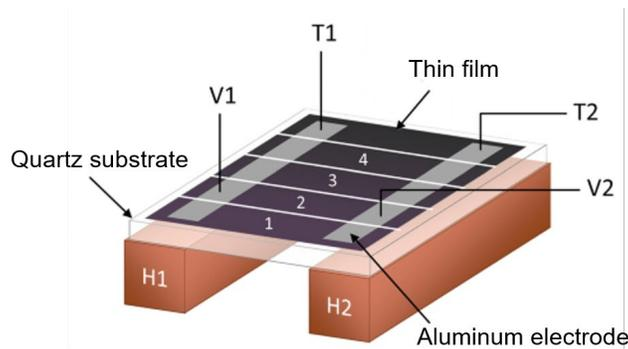
Figure 5: Schematic of the thermopower measurement system.
