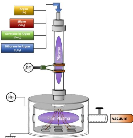
Figure 3: Schematic of the dual plasma co-deposition reactor for amorphous/nanocrystal film fabrication.
