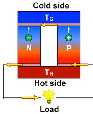
Figure 1: Schematic of a thermoelectric energy generator.
