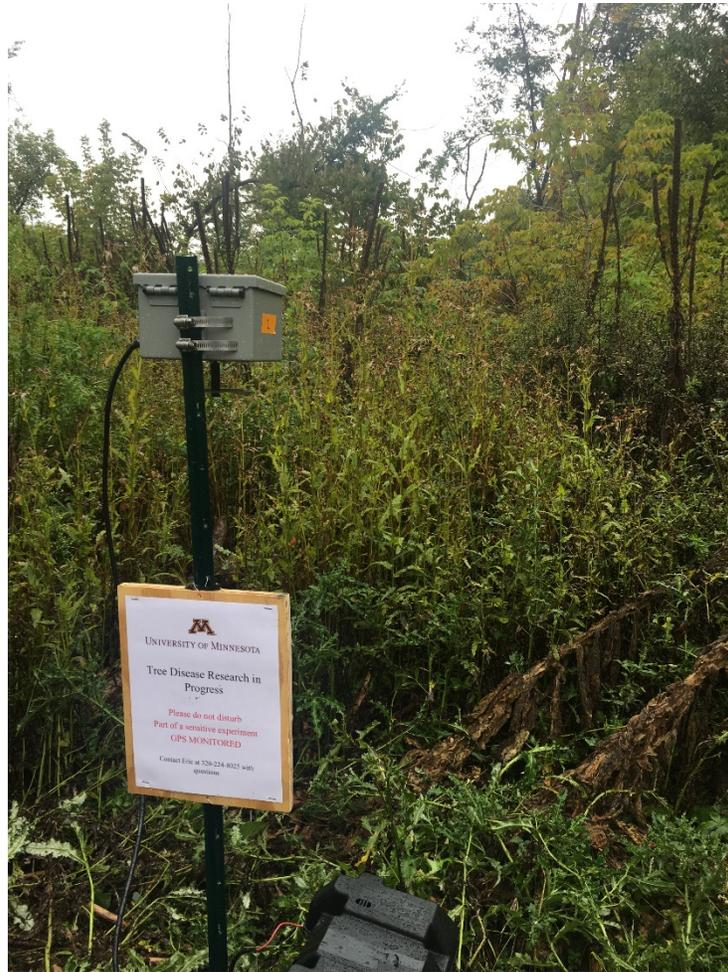
Figure 10. A rotation impactation sampler deployed in Minnieska, Minnesota.
