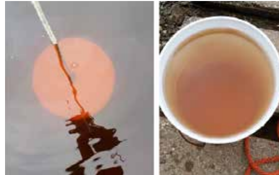
CDOM can be measured from 1) smartphone photos of a Secchi disk placed at a fixed depth in lakes, or 2) from photos of white buckets filled with lake water.
