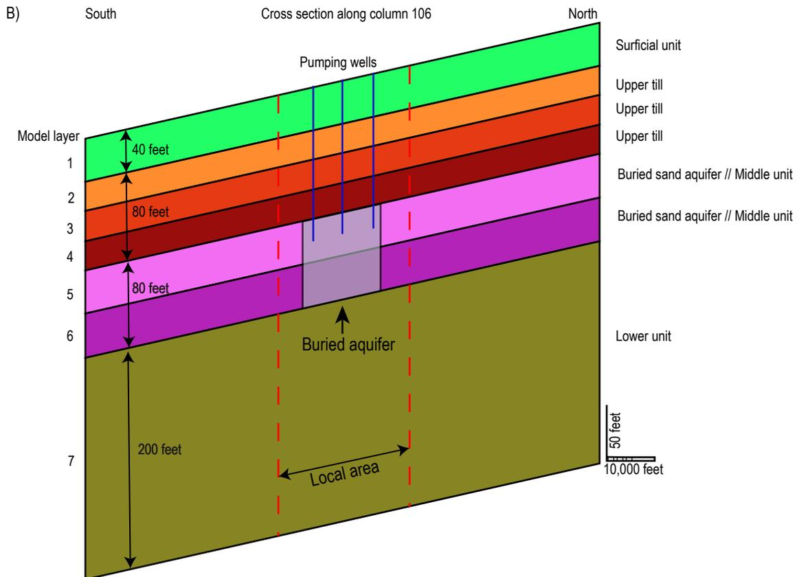
Figure 10: Interpretive model layout (A) top view and (B) cross section view.
