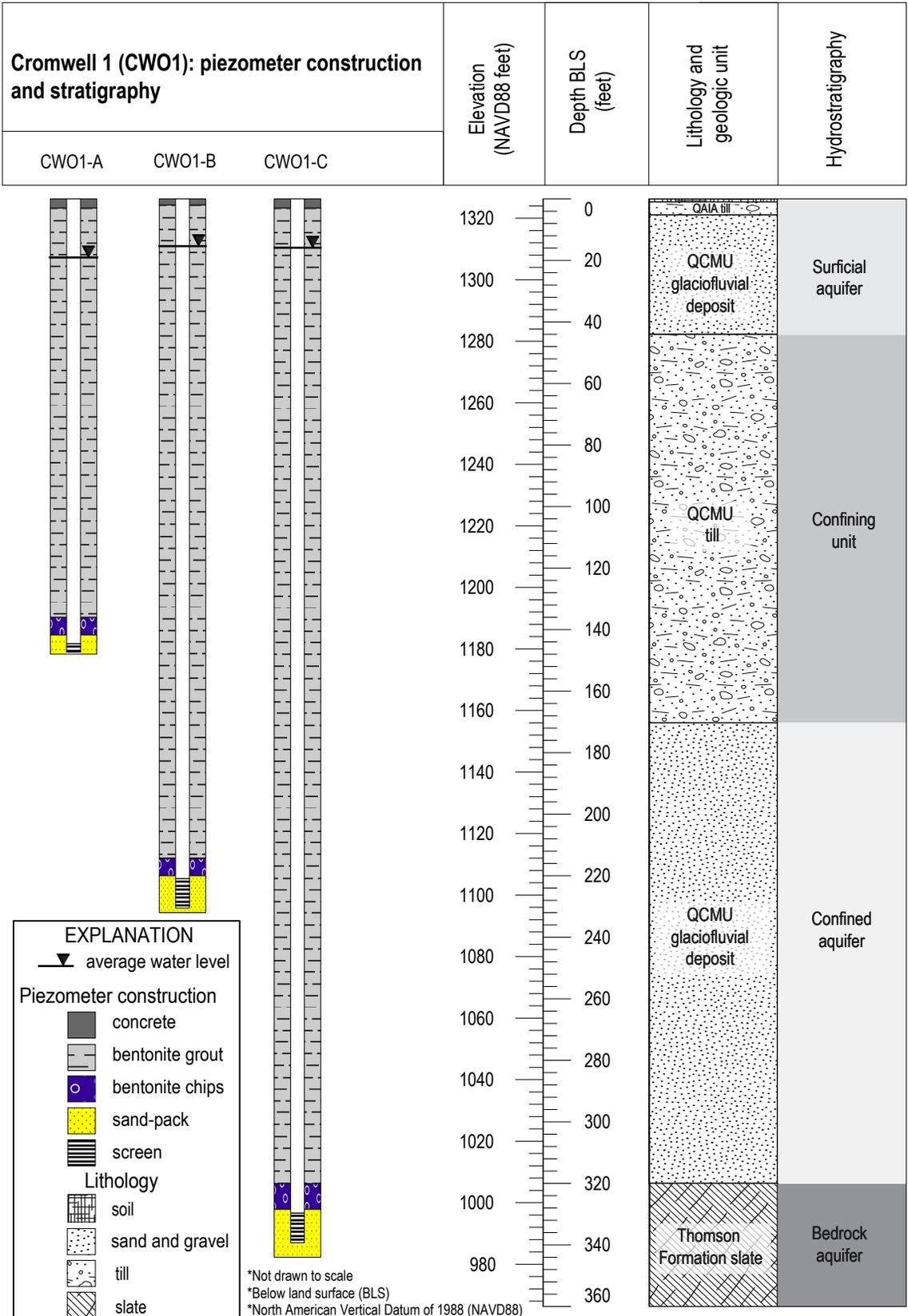
Figure 4: Stratigraphic information based on the Minnesota Geological Survey analysis (Staley and others, 2018) and Knaeble and Hobbs (2009). Unit abbreviations are as follows: QAIA, Alborn Member of the Aitkin Formation; QCMU, Cromwell Formation.
