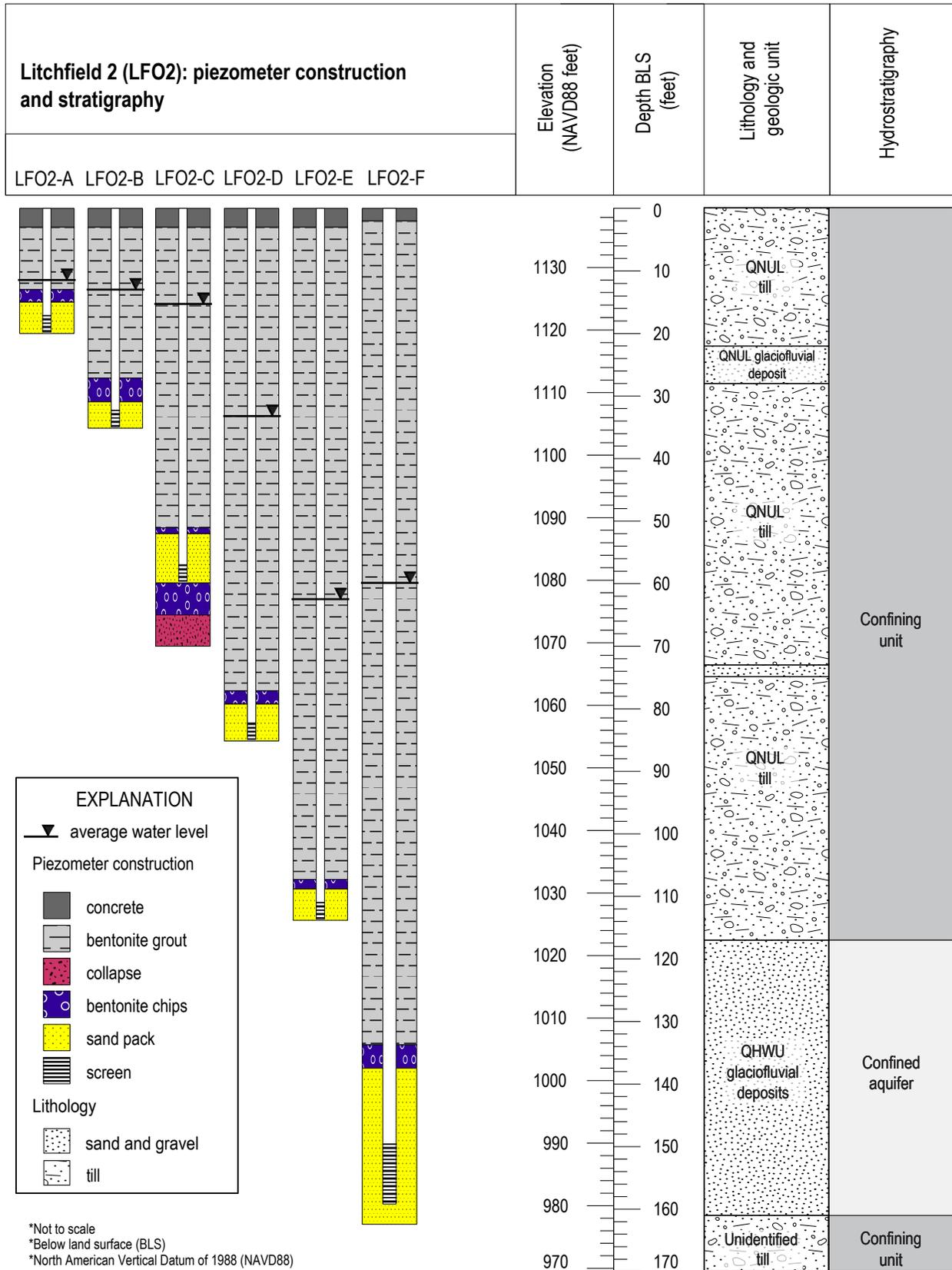
Figure 3: Stratigraphic information based on the Minnesota Geological Survey analysis (Wagner and Tipping, 2016; Staley and others, 2018). Unit abbreviations are as follows: QNUL, Villard Member of the New Ulm Formation; QHWU, Hewitt Formation.
