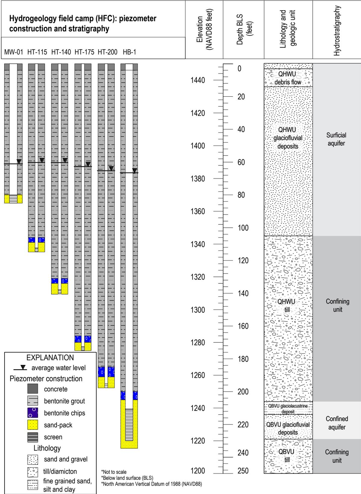
Figure 7: Stratigraphic information based on the Minnesota Geological Survey analysis (Staley and others, 2018). Unit abbreviations are as follows: QHWU, Hewitt Formation; QBVU, Browerville Formation.
