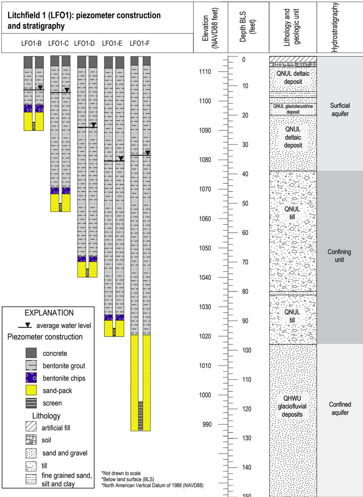
Figure 2: Stratigraphic information based on the Minnesota Geological Survey analysis (Wagner and Tipping, 2016; Staley and others, 2018). Unit abbreviations are as follows: QNUL, Villard Member of the New Ulm Formation; QHWU, Hewitt Formation.
