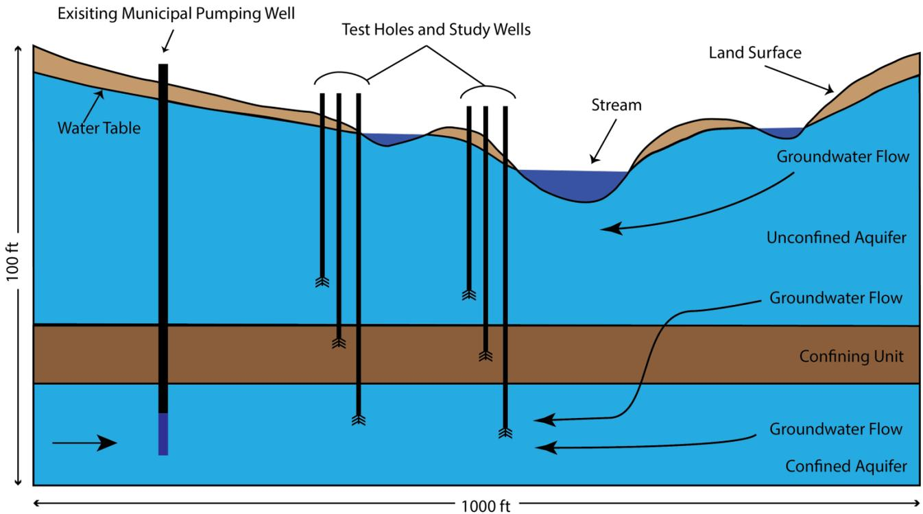
Figure 2. Expected well and piezometer installation site plan
