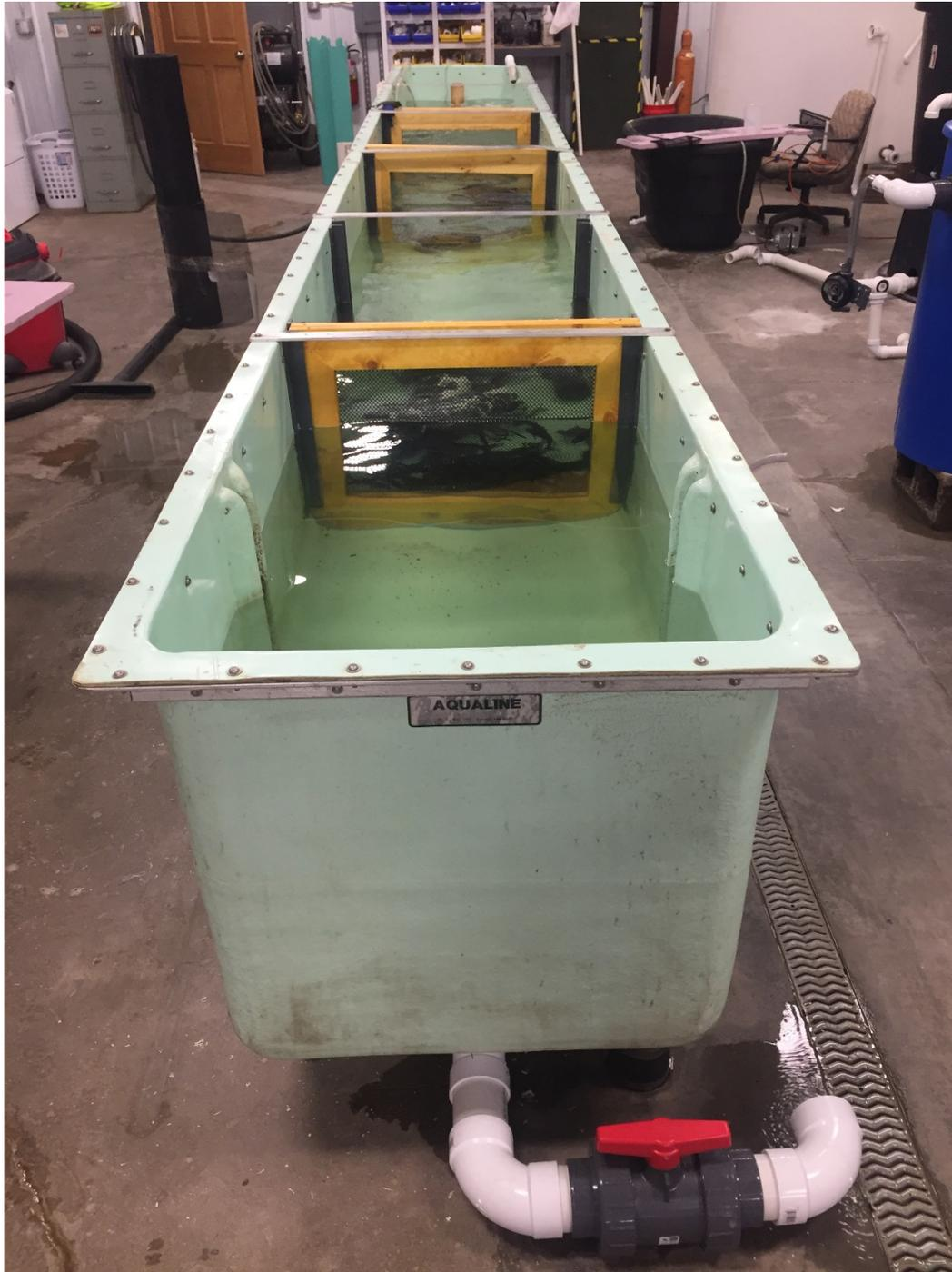
Figure 11. 30-foot flow through raceway, modified with compartments, used to hold host fishes such as Channel Catfish, Largemouth Bass, and Walleye.
