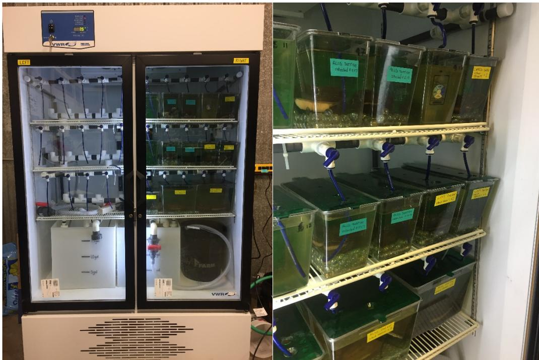
Figure 2. Laboratory refrigerator for mussel broodstock. Collected gravid females are held at 6°C to prolong the period over which the mussels will retain their glochidia. System was constructed in June 2017.
