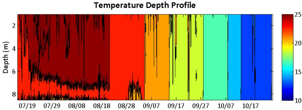
Figure 2. Temperature measurements in Madison Lake, MN, 2016. The color legend indicates water temperature in degrees Celsius. The y-axis is water depth starting at the lake surface and the x-axis is time.
