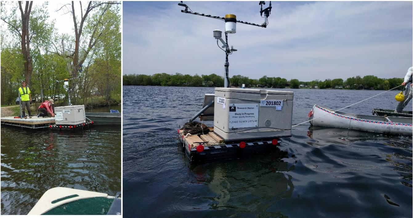
Figure. The cyanobacterial profiler with meteorological sensors, traversing stepper motor, and solar panel at the Ramsey Lake. The profiler was deployed on May 17<sup>th</sup>, 2018.
