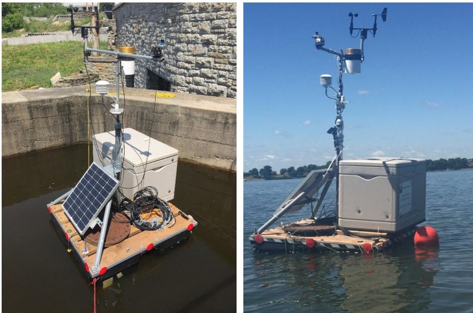
Figure. The proposed cyanobacterial profiler with meteorological sensors, traversing stepper motor, and solar panel. Left: Design and testing procedure at the St. Anthony Falls Laboratory. Right: The profiler deployed in Madison Lake, MN, on June 14, 2016.
