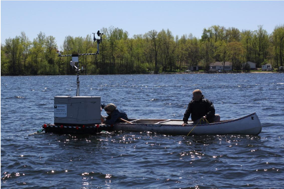
Figure. The cyanobacterial profiler with meteorological sensors, traversing stepper motor, and solar panel at the South Center lake. The profiler was deployed on May 18<sup>th</sup>, 2017.
