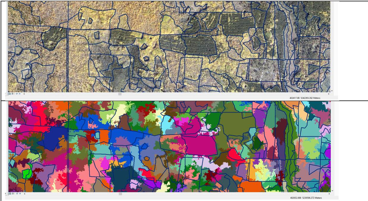
Figure 5. DNR managed FIM stands overlaid on CIR imagery (top) and on the stand segments (below) produced from LiDAR.
