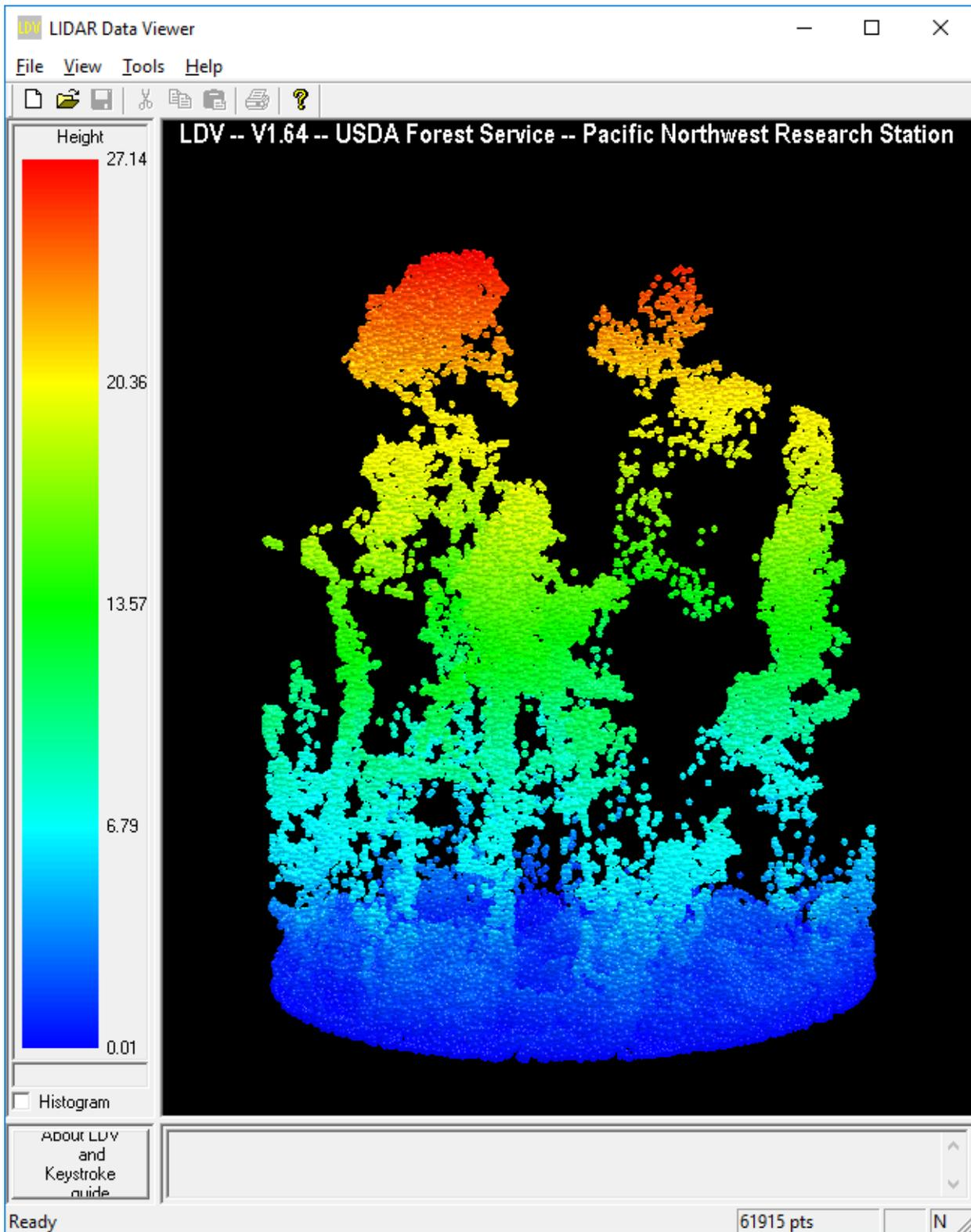
Figure 2. LIDAR point cloud clipped for one of the plots measured in summer 2018.
