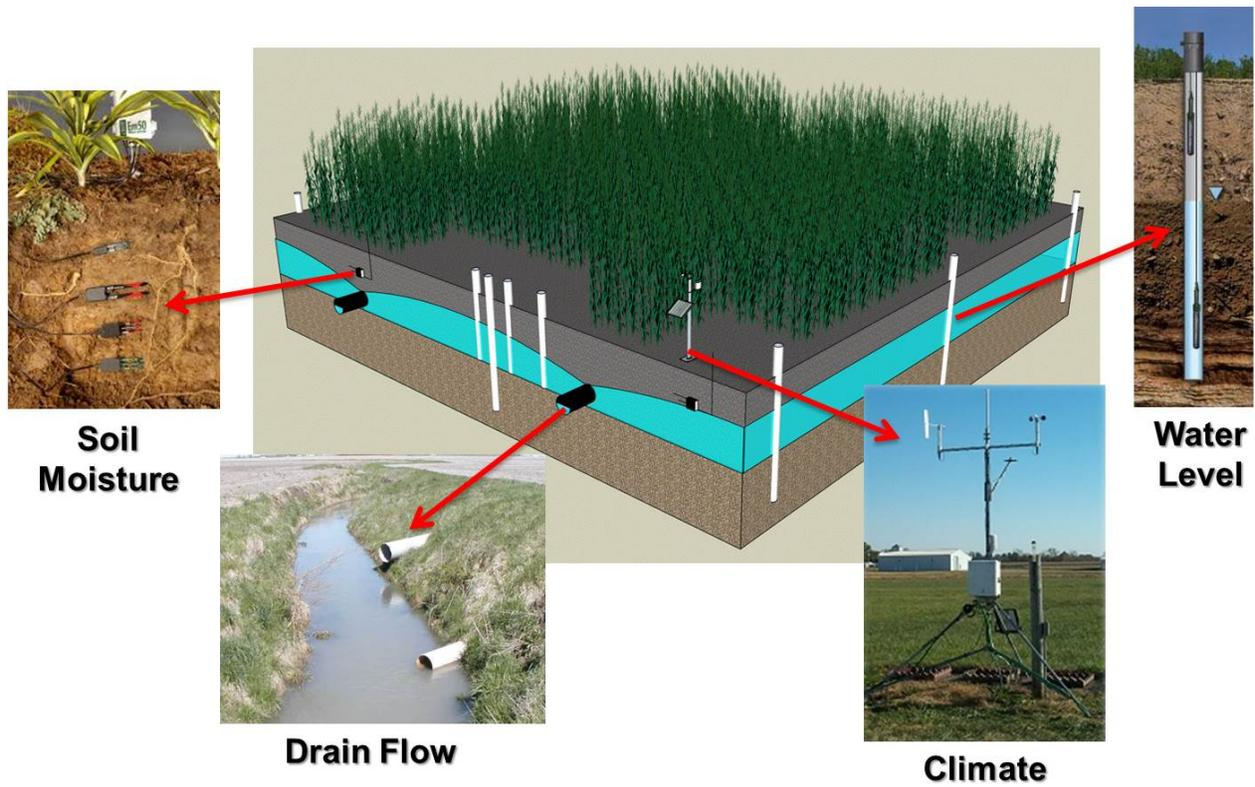
**Figure 2.** A hypothetical configuration of one of the two drained field sites, including a weather station for measuring climate data, a piezometer network for continuous water level measurements, soil moisture probes, and subsurface drainage flow. The third undrained field site will have a similar configuration, with the absence of subsurface drainage flow.
