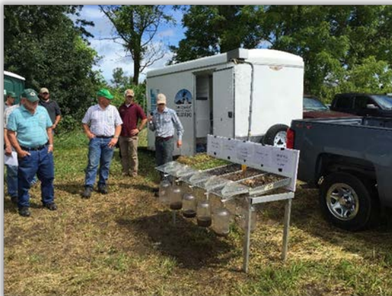
Rainfall simulator in use at the field day in Eyota.
