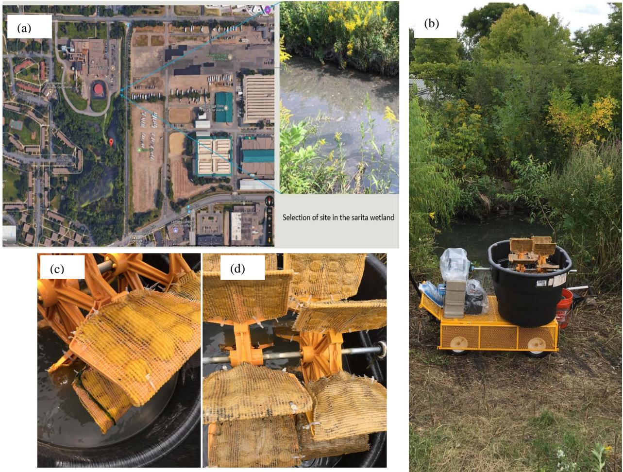
**Fig. 18** (a) Location of the Sarita wetland (b) Paddle wheel reactor onsite for the nutrient recovery (c) Biofilm on the paddle recovering P,N and COD in Sarita wetland and the (d) biofilm after 7 days of
