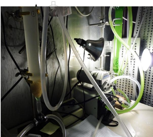
**Fig. 15** Schematics and picture of the flow through design reactor for nutrient recovery
