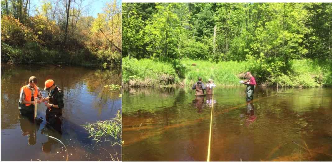
Figure 1A: LEFT: CTD and turbidity sensor installation at the downstream site. RIGHT: Dr. Rose with students collecting stream-cross section measurements to accompany sensor installation.
