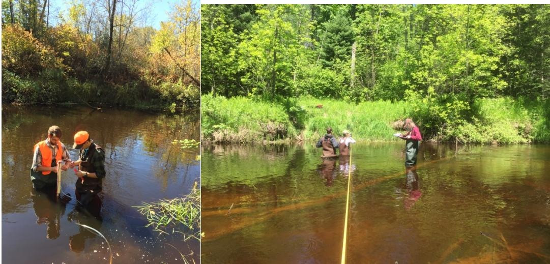
Figure 1A: LEFT: CTD and turbidity sensor installation at the downstream site. RIGHT: Dr. Rose with students collecting stream-cross section measurements to accompany sensor installation.
